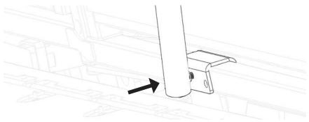
**3** Insert the clipping rail into the top bracket.
