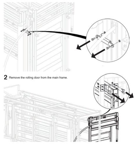
${\bf 3}\,$  Remove the rolling door track plate, and switch to the opposite side.
