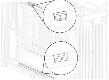
2 Attach the trimming bar to the bottom bracket.
