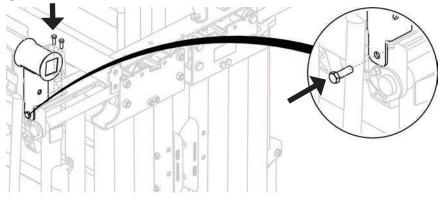
7 Flip the axle pin on the rear control bracket and transfer it to the opposite side.
