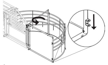
2 Connect top joiner bars A, B, and C to panels 1, 2 and 3 as shown. TIP: Lower the unit to line up top joiner bars with panels
