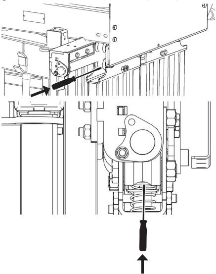
**4** Tilt the screwdriver/pry bar up and into the head gate roller. This will push down the spring, releasing the locking mechanism on the head gate door.
