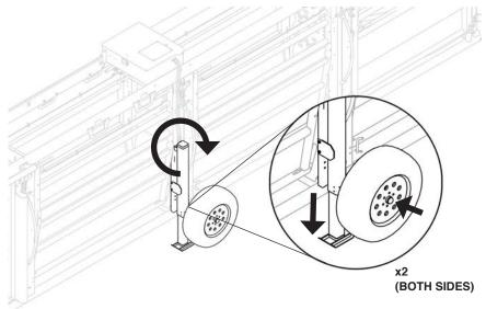
**3** Retract rear jacks using **DOWN** button / rear jack handle until they stop.
