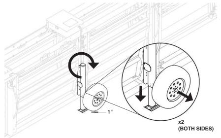
8 Retract rear jacks to set the unit on the set the unit on the ground until they stop using **DOWN** button / rear jack handle.
