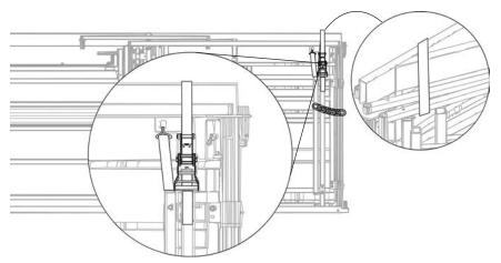
5 Retract the bottom joiner bar and secure with the pin.
