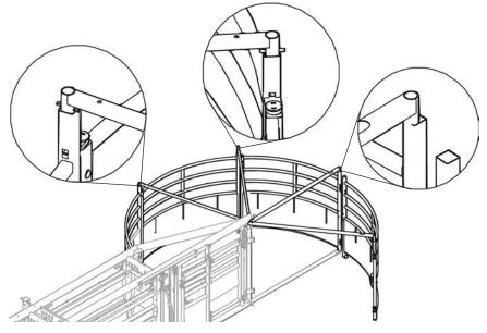
**5** Fold out the 3E door and secure with joiner bar E. Set aside transport pins.
