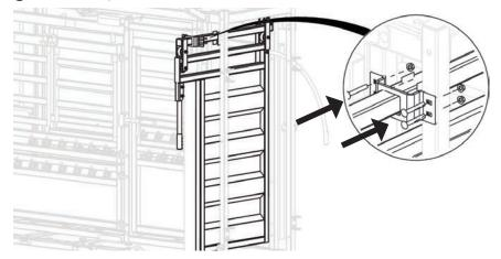
6 Install the rolling door handle slider on the right-hand side.
