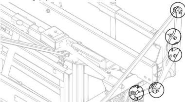
b. You should feel the head gate rollers moving when you open the head gate. The rollers should be tight enough to be moved by hand, but not over-tight to cause the rollers to bind.
