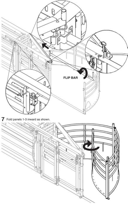
17 | TRANSPORTING THE Q-CATCH 87 SERIES PORTABLE WORKING SYSTEM
