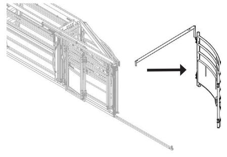
2 Unfold panels 1-3 and attach to the bottom joiner bar.
