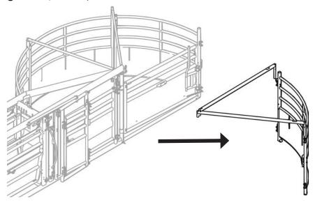
4 Latch the swing gate to the left-hand side of the rolling door.
