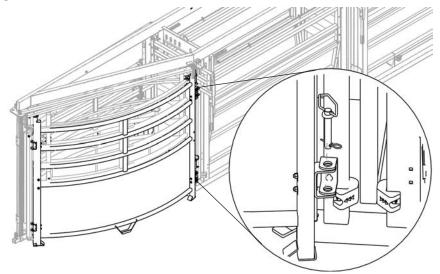
**9** Secure the panels with the ratchet strap and transport chain as shown.
