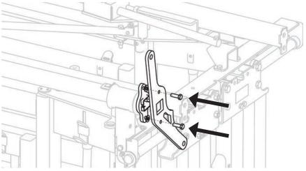
Install the head gate hammer and connect it to the squeeze arm plate.
