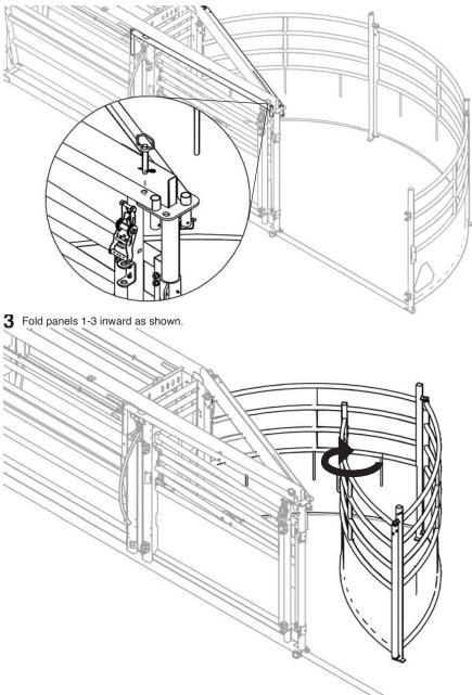
4 Secure the panels with the ratchet strap and transport chain as shown.
