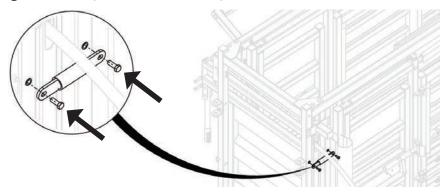
7 Remove the rolling door lock and move to the opposite side.
