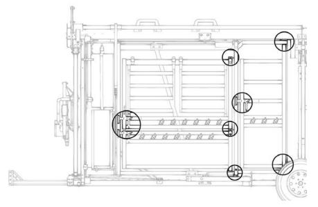
✓ Check gate latches and striker plates for wear. Ensure gates are locking securely.
