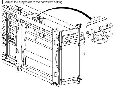
2 Lift the side panel and set the latch above the alley bow. Repeat step for the opposite side panel.
