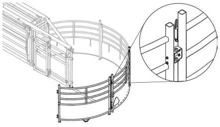
4 Connect top joiner bars A, B, C, & D to panels 1, 2, 3 and 4 as shown. TIP: Lower the unit to line up top joiner bars with panels
