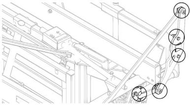
b. You should feel the yoke gate rollers moving when you open the yoke gate. The rollers should be tight enough to be moved by hand, but not over-tight to cause the rollers to bind.
