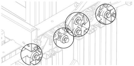
✓ Clean bottom yoke gate door track to prevent dirt-build-up.
