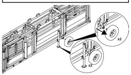
**6** Using both jacks simultaneously, lower the unit until the forcing pen section is 3-6" above the ground.
