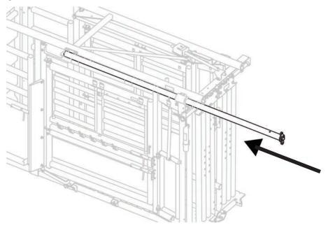
**9** Insert the Q-Catch handle and mount the control tube on the rear control bracket. Secure with a bolt on the opposite side.
