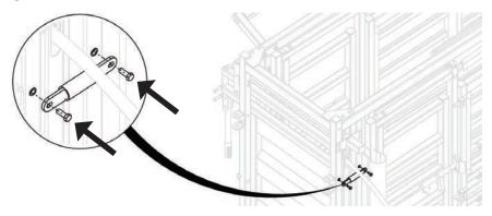
7 Remove the rolling door lock and move to the opposite side.
