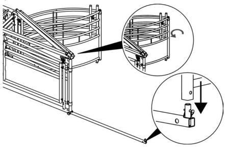
Attach the top joiner bars to the panels as shown.
