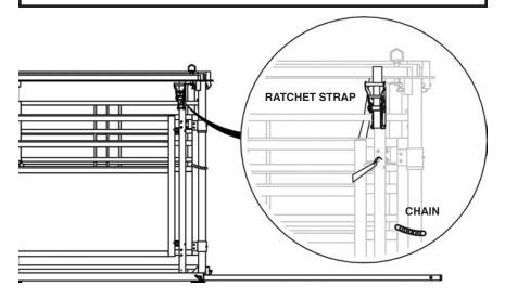
TRANSPORTING THE Q-CATCH 74 SERIES MOBILE WORKING SYSTEM | 6
