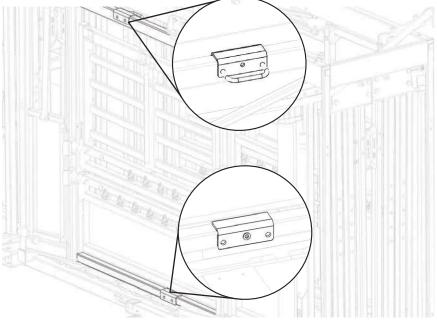
**2** Attach the clipping rail to the bottom bracket.
