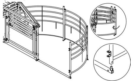
**5** Secure panels with the ratchet strap and transport chain as shown. Tighten the ratchet strap to prevent sag in panels during transport.
