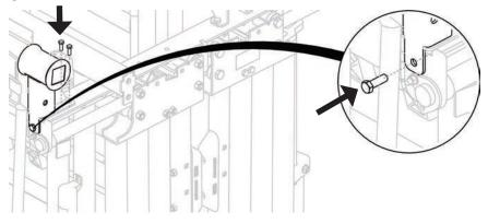
7 Flip the squeeze axle welding on the rear control bracket and transfer it to the opposite side.
