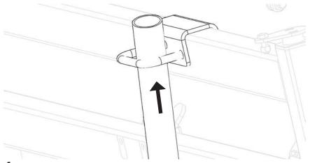
4 Adjust clipping rail position to your preference. Tighten bolts to secure.
