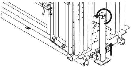
4 Transfer the front jack to the race section. At this point, both jacks should be attached to either side of the race.
