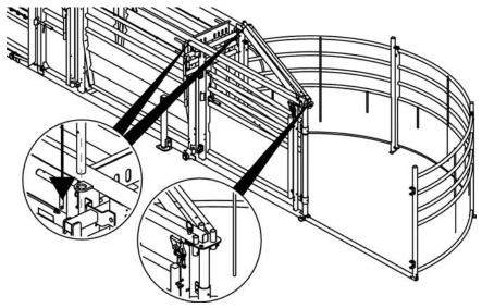
**3** Using both jacks simultaneously, raise the unit until the forcing pen section is 3-6" above the ground.
