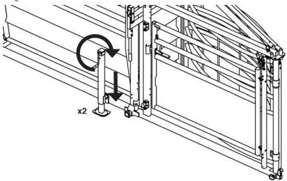
7 Remove the pin and pull out the bottom joiner bar. Secure with the same pin.
