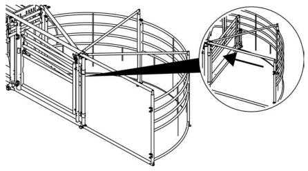
2 Return the top joiner bars to their respective holders. Secure the top left joiner bar with the pin.
