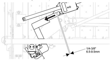
d. Apply outward pressure on the squeeze handle. Adjust the front bolt until the fandangle presses the lock box release pin 1/4" - 3/8" in towards the lock box, which will release the lock mechanism and allow the squeeze to open fully.
