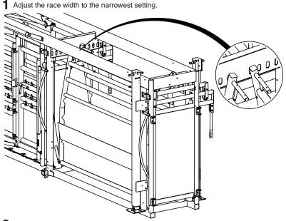
2 Lift the side panel and set the latch above the race bow. Repeat step for the opposite side panel.
