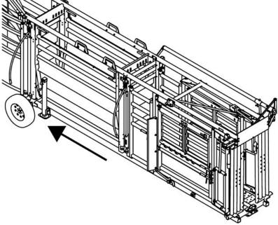
**5** Using both jacks simultaneously, raise the unit until the tires are 1" above the ground. Remove tires and set aside.
