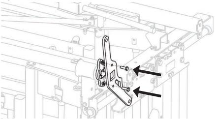
Install the yoke gate hammer and connect it to the squeeze arm plate.
