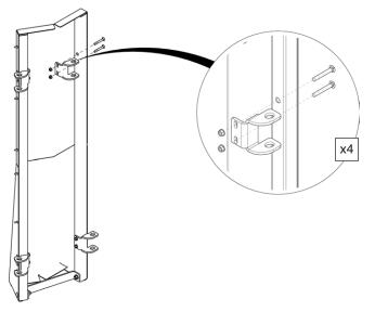
5 Connect the Kicker Panel to the Easy Flow Cattle Alleys to form the outside of the curve.
