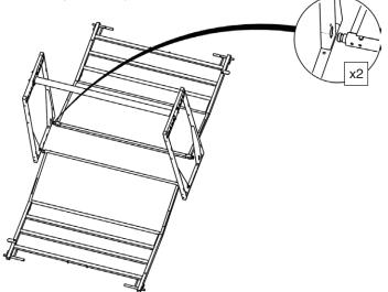
5 Insert the bottom pins on the panel into the frame on the opposite side.
