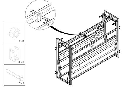
**3** Install the chain clip and secure to the centre bar on the Alley Stop.
