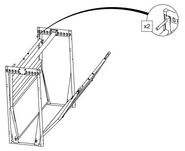
7 Connect to chute, alley or other equipment using the provided panel pins.
