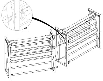
**3** Connect the two alleys together on the side that you want to form the inside of the curve using 2 panel pins.
