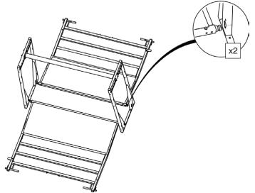
6 Lift the panels up and latch into the frame. Tighten all fasteners to secure.
