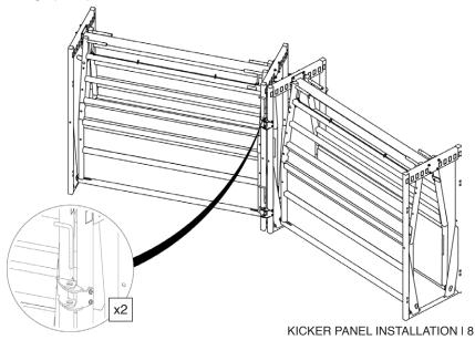
4 Move the Panel Clips on the Kicker Panel into the correct position.
