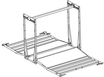
**4** Insert the bottom pins on the panel into the frame on one side.
