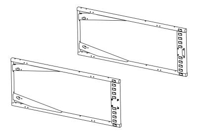
**2** Install the top post in the alley. Keep nuts loose.
