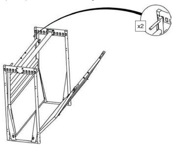
**7** Connect to crush, race or other equipment using the provided panel pins.
