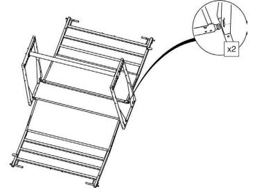
6 Lift the panels up and latch into the frame. Tighten all fasteners to secure.
