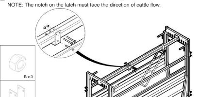
3 Install the chain clip and secure to the centre bar on the Race Stop.
