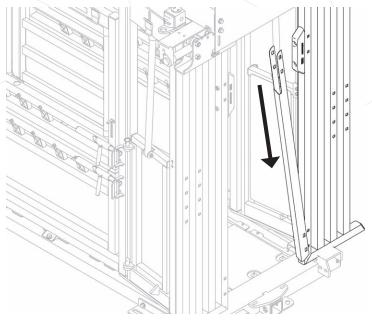
4. Secure Left-Hand Bull Catcher Sheet Metal on the Yoke Gate Door with 4x Carriage Bolts and 4x Flange Nuts.
