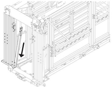
6. Secure the Right-Hand Bull Catcher Sheet Metal on the Yoke Gate with 4x Carriage Bolts and 4x Flange Nuts.
