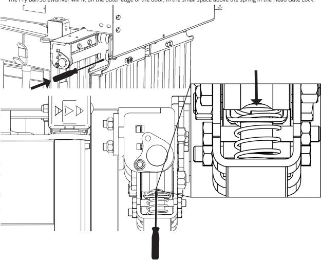
3. Tilt the Pry Bar/Screwdriver up and into the Head Gate roller. This will push down the spring, releasing the locking mechanism on the Head Gate doors.
