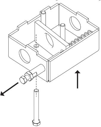
6. Slowly release pressure on the lock plate and remove the lock plate, spring, and small shaft from the mechanism.
