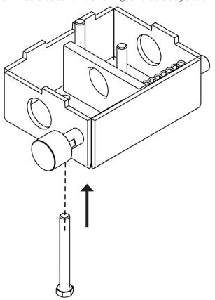
10. Slowly release pressure on the lock plate and remove the lock plate, spring, and small shaft from the mechanism.
