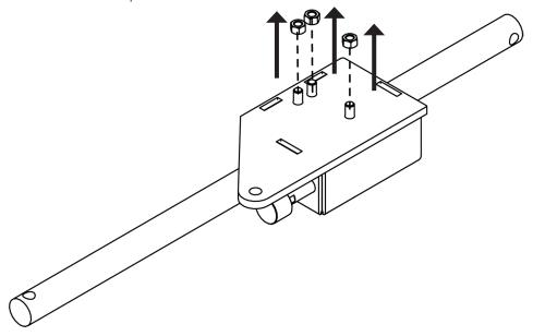
7. Remove the back plate to expose the locking mechanism.
