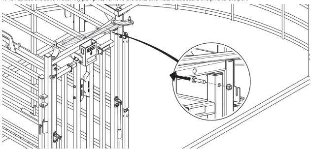
2. Pull the pins up and out. If the pins do not come out, they may need to be cut at the red line shown in the image below.
