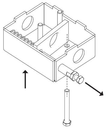
6. Slowly release pressure on the lock plate and remove the lock plate, spring, and small shaft from the mechanism.
