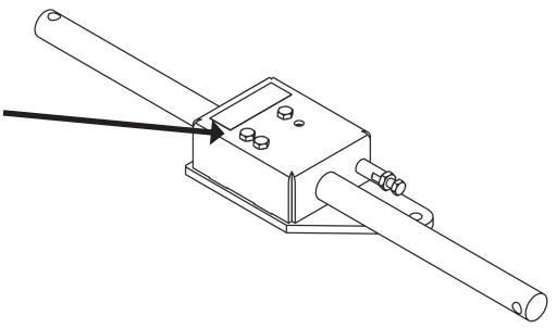
2. Turn the lockbox upside down and remove the three nuts.
