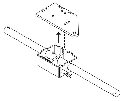
4. Push the lock pin, pushing the lock plate towards the two bolts, and remove the long lock shaft. **NOTE: Shaft can be removed through either end of the lockbox.**
