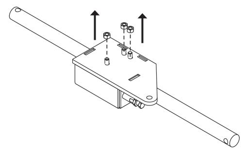
3. Remove the back plate to expose the locking mechanism.
