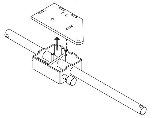
8. Push the lock pin, pushing the lock plate towards the two bolts, and remove the long lock shaft.
