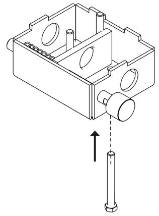
10. Slowly release pressure on the lock plate and remove the lock plate, spring, and small shaft from the mechanism.
