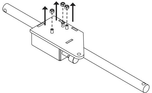
7. Remove the back plate to expose the locking mechanism.
