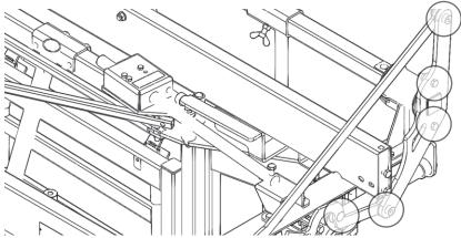
b. You should feel the yoke gate rollers moving when you open the yoke gate. The rollers should be tight enough to be moved by hand, but not over-tight to cause the rollers to bind.
