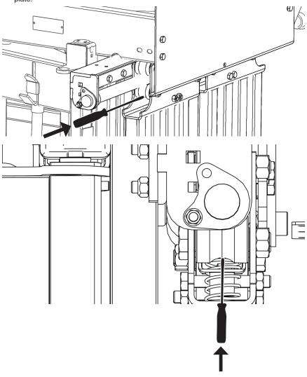
4 Tilt the screwdriver/pry bar up and into the yoke gate roller. This will push down the spring, releasing the locking mechanism on the yoke gate door.
